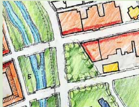
The sketch depicts a new park where the other sketch shows the bell tower site. This sketch also directs primary traffic along a new route adjacent with the railroad tracks, while First Avenue would become a more local-serving street, ending at a "T" intersection at its northerly terminus.
